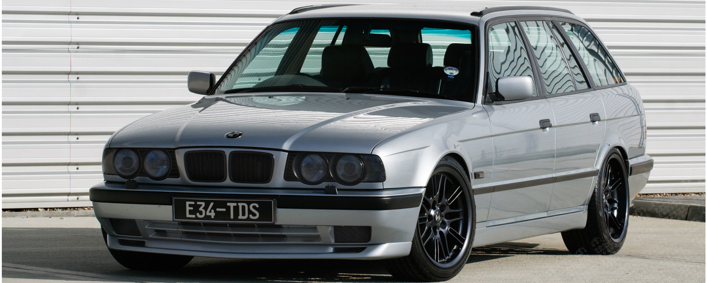
Tommy's e34 525 tds Touring with 18" E39 M5 Alloys 8.5x18 front 9.5x18 rear, Lowered suspension, M5 Front/rear bumper, M5 door kick-panel trim, De chromed front grill, Smoked Front > Light/indicators, All Red Rear Lights, 55w 6000k Hid, Carbon Badges all round, Custom exhaust system, Dark Grey Leather interior with front Elec memory Recaro's, Piano Black trim >>>>
