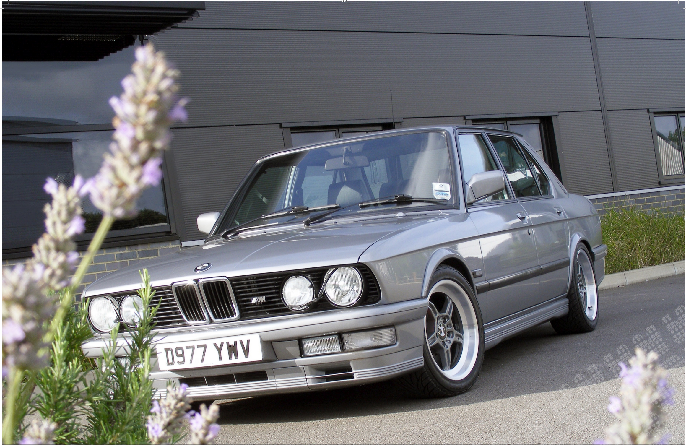
Sepia's 1987 E28 M535i 5 spd manual in Lachs Silver, 87,000 miles, Black leather sport interior, Shadowline, Custom made suspension springs, 355mm front discs & AP Racing 4 pot calipers, E34 540 rear discs and calipers, Hartge strut brace, Whiteline anti-roll bars, Fritz s/s exhaust system, 17" colour coded throwing star alloys, winner of 'Best e28' at Bimmerflex 2009 >>>>
